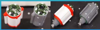
Figure 3. Scaled SL-8 rocket bodies used for OMC study. Orange/white color scheme is used to model commercial missions, while gray paint scheme best reflects Russian government missions. The left image shows both models as seen from the payload end. The right image shows the side view, with thrust (primary rocket nozzle) pointing toward the lower-left.
