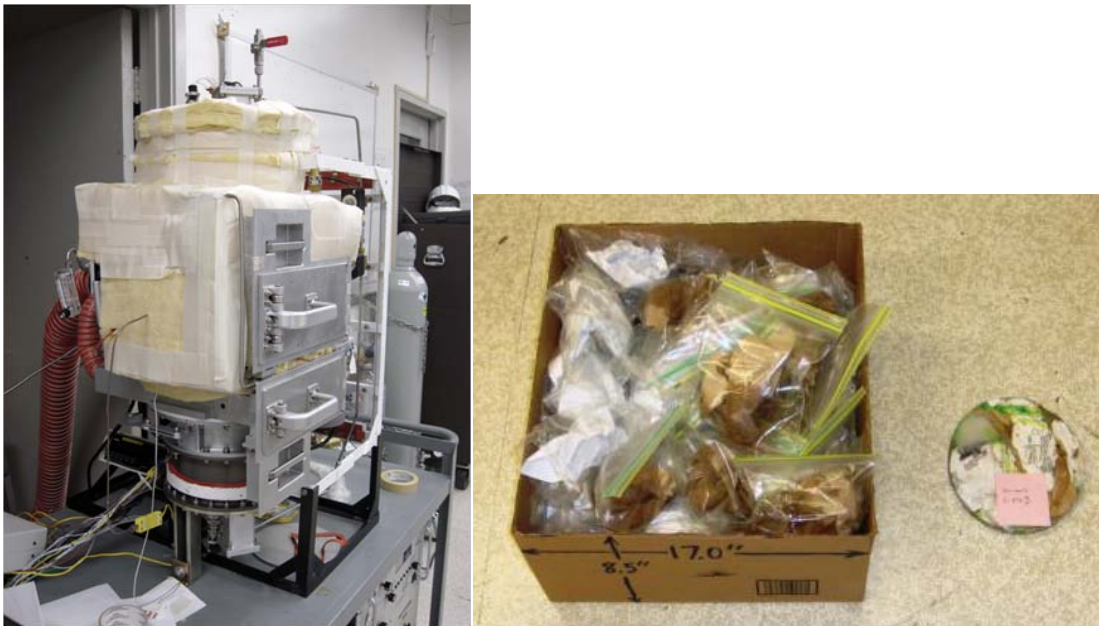
Figure 5. Left: first-generation HMC. Right: example of compaction of loose trash to a stable HMC tile.
