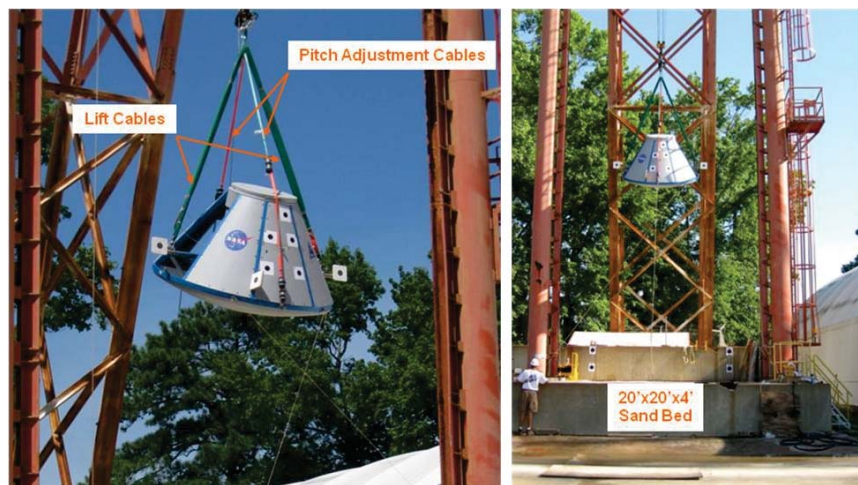
Figure 3. Vertical Drop Test Set-Up.
