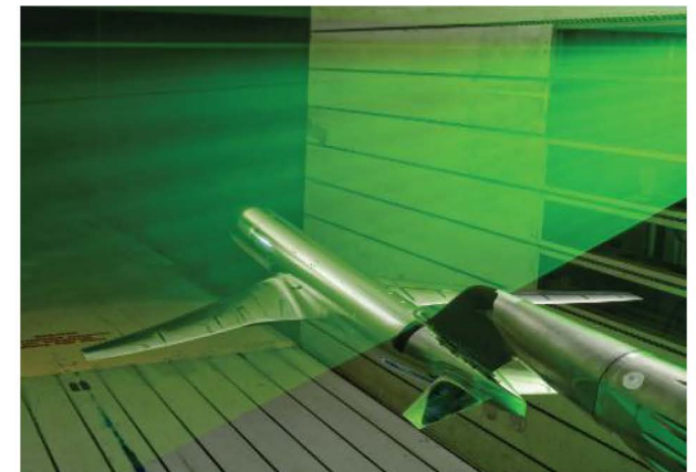
Particle Image Velocimetry in 11-foot
