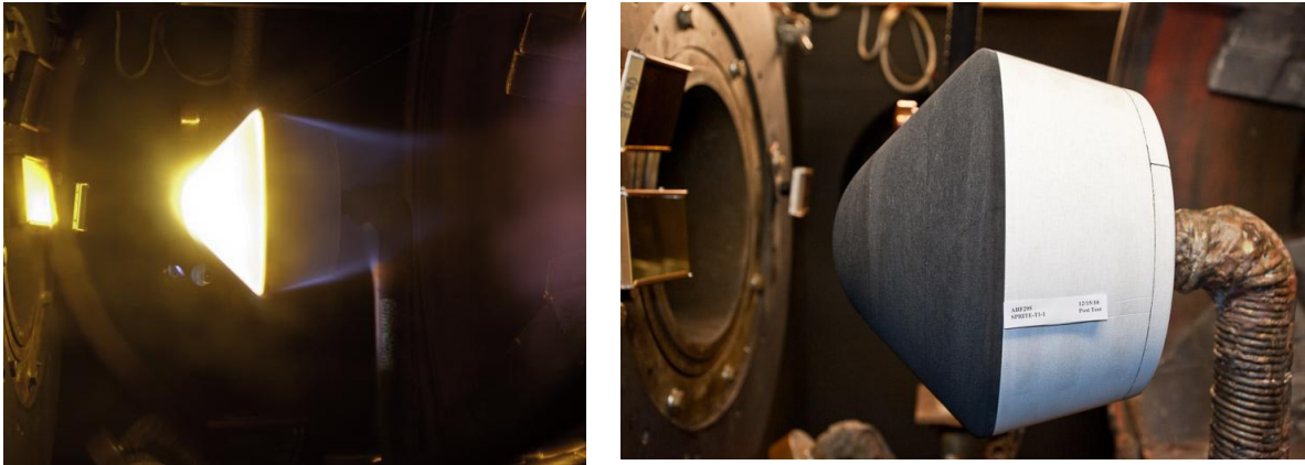
Figure 11: SPRITE model during and after the arc-jet tests.
