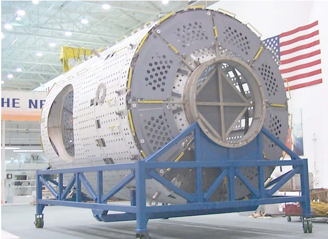
Figure 5: NBL Large Mockup Example - Node 2
