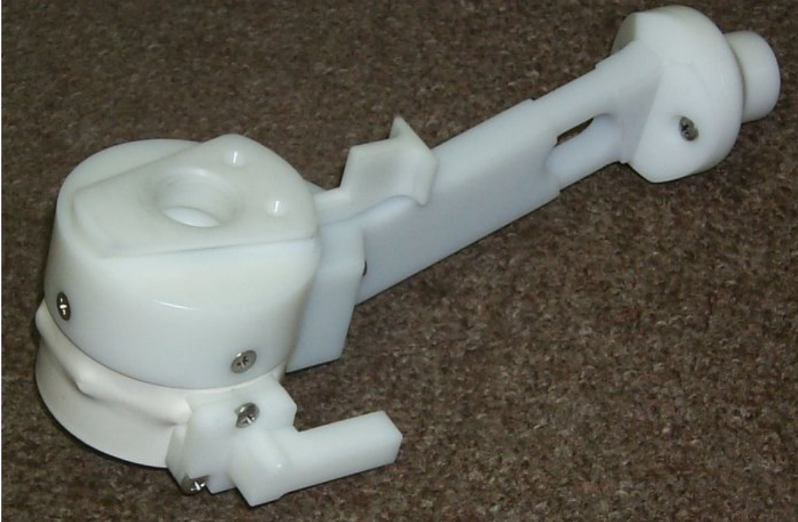
Figure 3: NBL Small Hardware Example - Neutrally Buoyant Round Scoop
