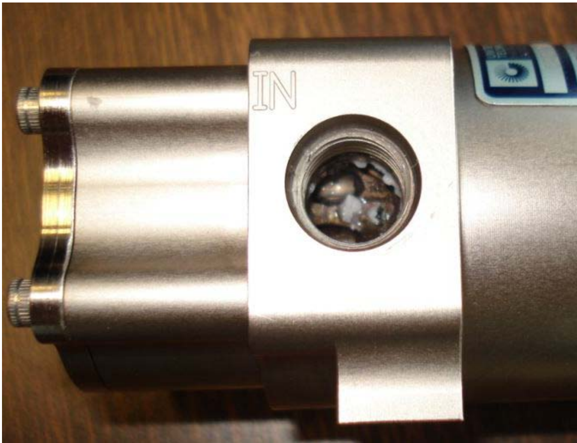
Figure 6. Corrosion products from the prototype aluminum housing are visible through the inlet port.
