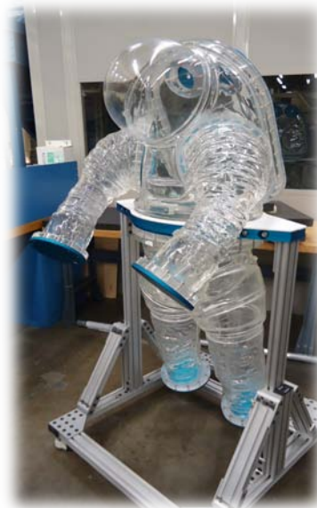
Figure 9. Space Suit Assembly Simulator
