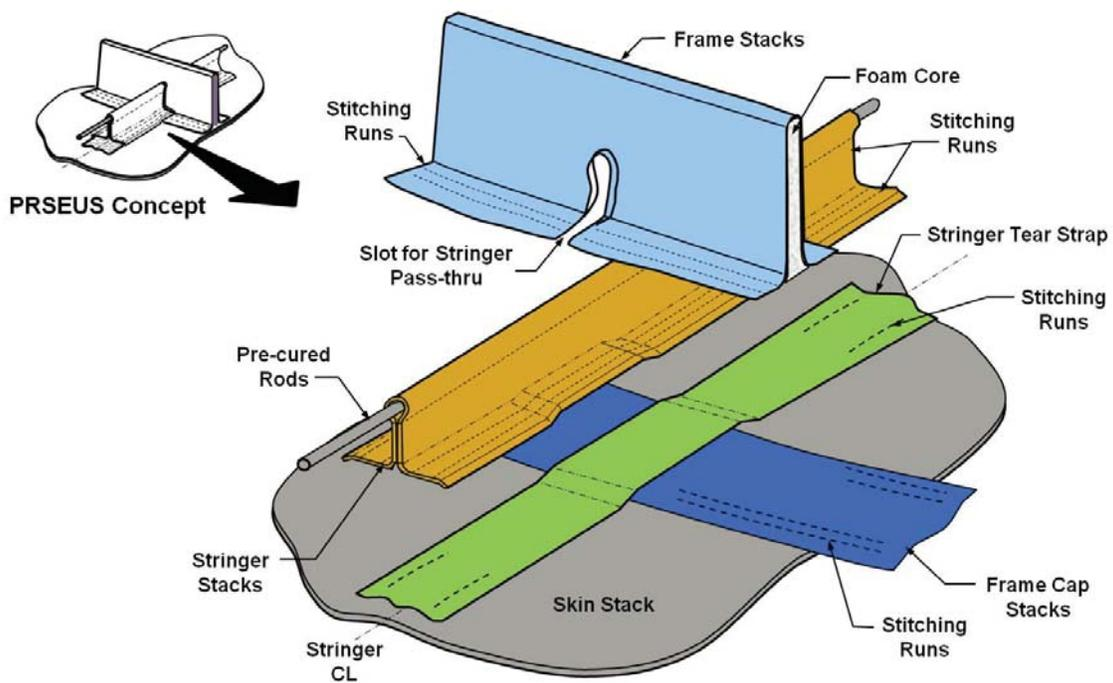
Figure 2. PRSEUS design concept baseline for the HWB.
