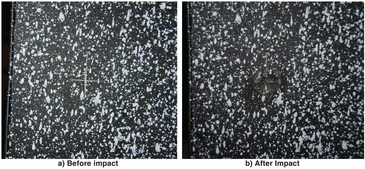
Figure 19. Impact location before and after impact.
