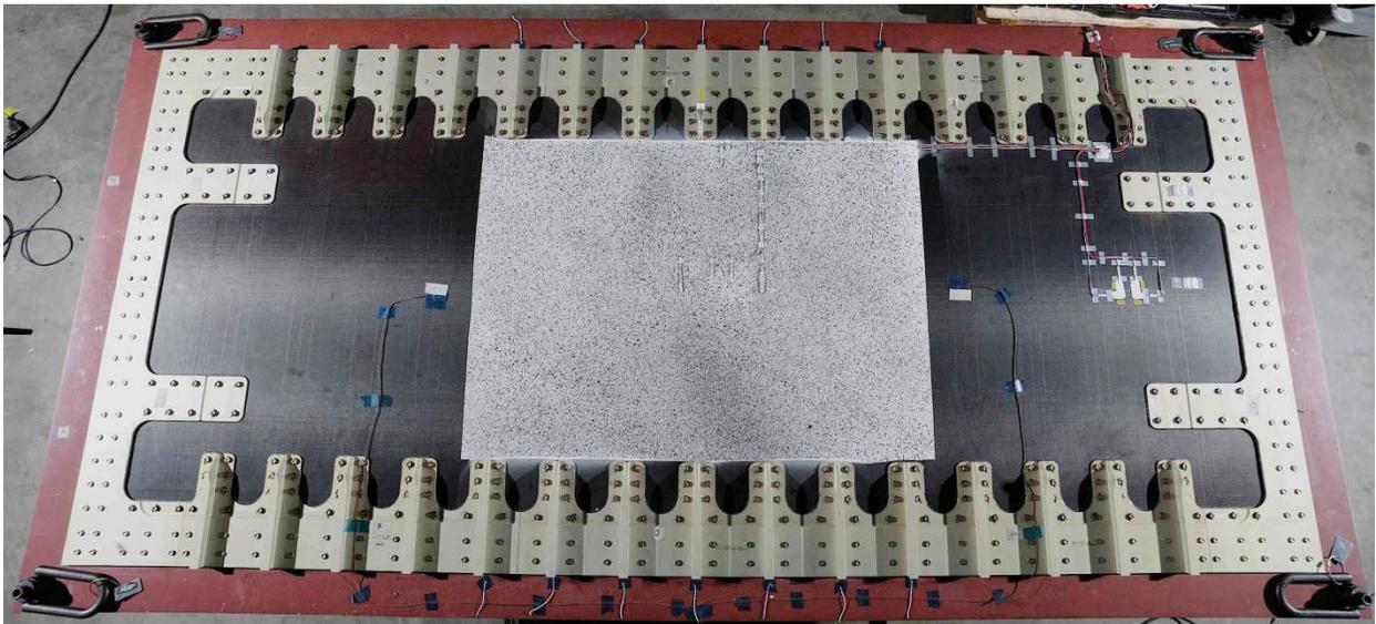
**Figure 5. Pressure panel test assembly. Doublers with integral stiffeners are the yellow structure around the perimeter of the panel. The VIC speckle pattern is the white region in the center, and measures approximately 29 by 40 inches.**
