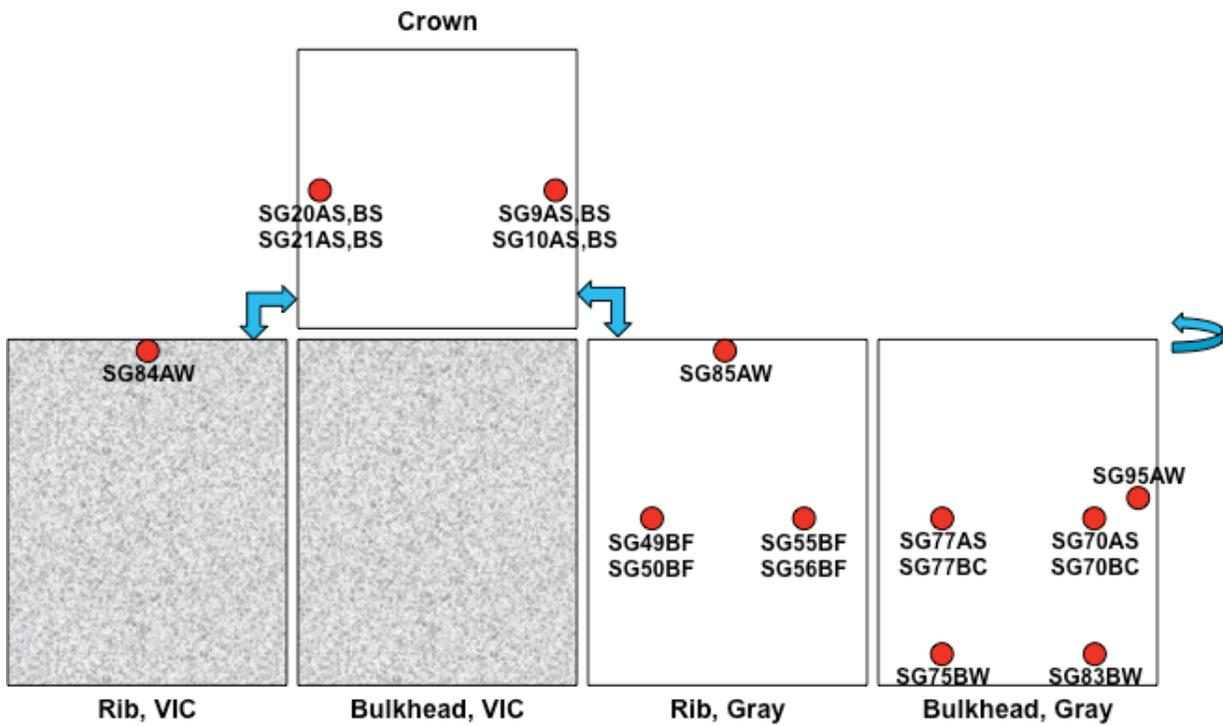
Figure 15. Strain gage locations. Details about locations are presented in table 2.
