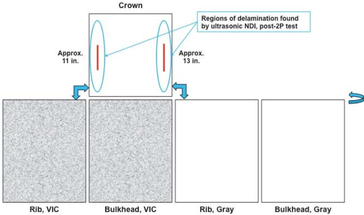
Figure 28. Delaminations discovered by NDI after loading up to 2.2P.
