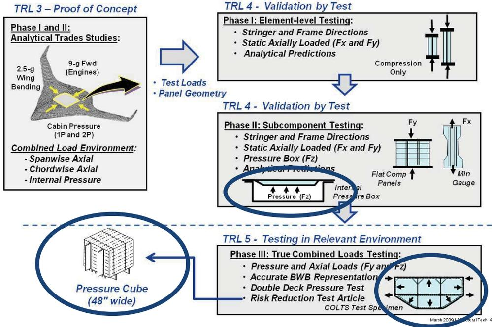
Figure 3. HWB structural development building block approach.
