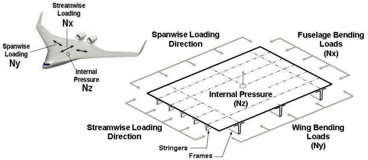
Figure 1. HWB conceptual vehicle and loading patterns.
