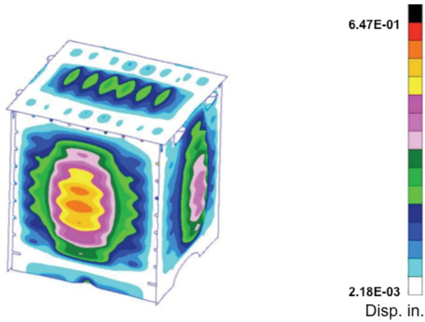
Figure 11. Nastran nonlinear analysis displacement contours at 28.5 psi
