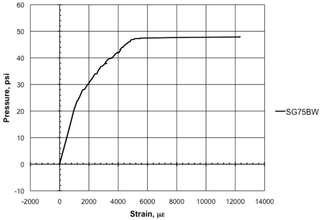
Figure 36. Strain measured at gage SG75BW during loading up to catastrophic failure.
