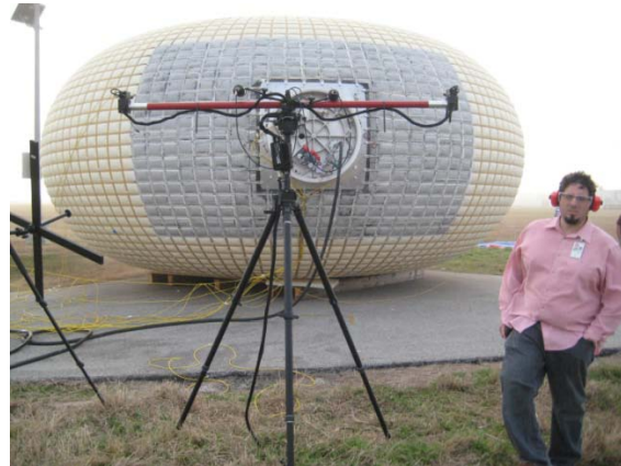
Figure 3. Phase II article with Painted “Dot” Pattern and Photogrammetry Camera System.
