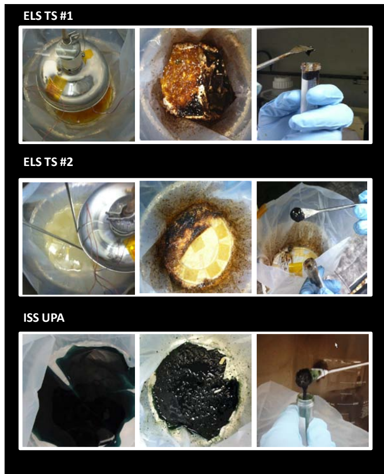
Figure 3. Examples of the single-batch brine drying process. Frames: Left to Right – brine influent, dried brine residual, collected solid sample.
