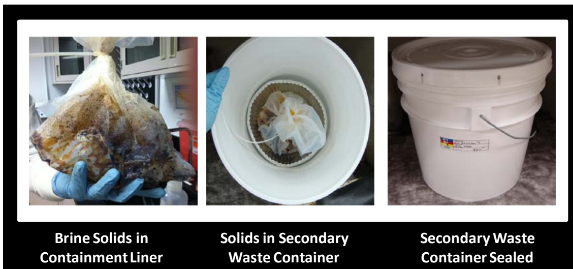
Figure 6. Examples of brine disposition during Multi-Batch Testing.
