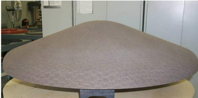
Figure 3 – 1.0-meter aeroshell with SRAM TPS
