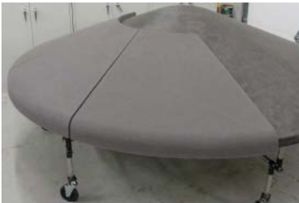
Figure 4 – Fit check of TPS modules on 2.65-m aeroshell.
