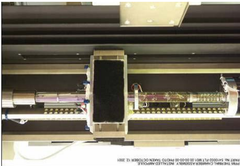
Internal View of PFMI Chamber Showing Sample
