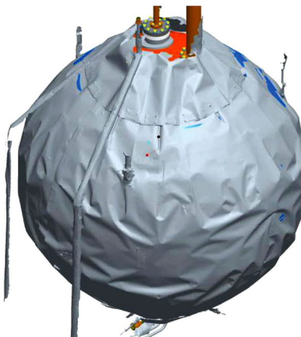
Figure 5.—Post test tank image with MLI outer shape sprayed with talcum powder, which the 3-D mapping tool needed to map the MLI. Notice the MLI ridges near the top, which reveal that the MLI substructure failed.
