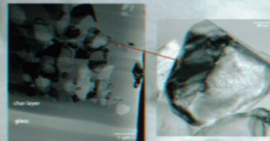
Figure 8. Bright field TEM image of Columbia window near the interface of the glass and char layer (left). Crystals were characterized based upon morphology, chemistry, and crystal structure (right) (NASA/KSC, UCF).
