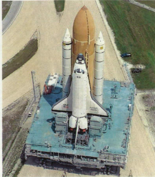
Figure 2 - MLP Transporting the Space Shuttle
