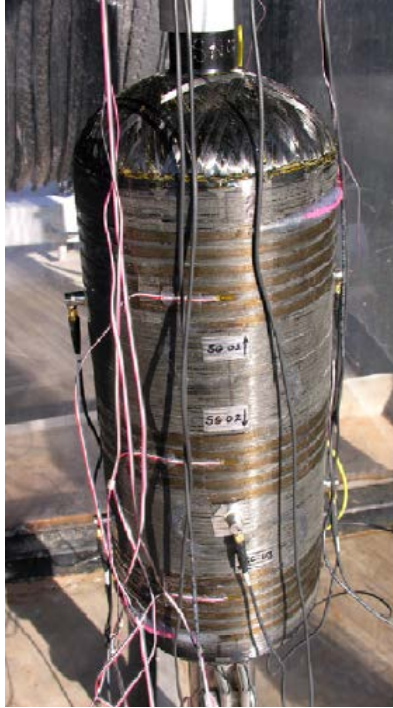
Figure 2. Second generation ‘smart’ composite overwrapped pressure vessel with circumferential fiber Bragg grating arrays on the top, center, and bottom of the cylindrical section, strain gages, and wideband acoustic emission sensors.
