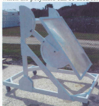
Figure 1: Solar concentrator used in sintering experiments at KSC.
