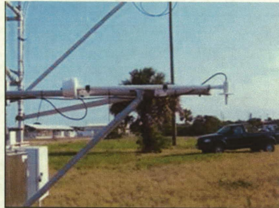
Figure 3. A mechanically aspirated 1.8 m temperature sensor at tower ID#0403.
