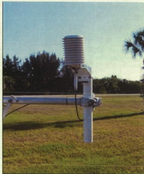
Figure 4. A naturally aspirated 1.8 m temperature sensor with radiation shield at tower ID#1007.
