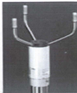
Figure 3. Image of the ultrasonic type RSA wind sensor mounted on the 10 towers used in this study (Vaisala Model WS425 Ultrasonic Wind Sensor). See Vaisala (2004) for details. Wind speed accuracy is \pm 0.26 kt or 3% of wind speed, whichever is greater. The starting threshold is virtually zero.
