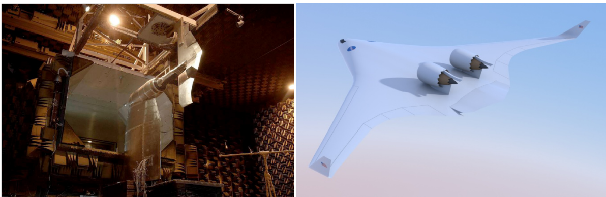
Figure 13.—NASA/Boeing propulsion aeroacoustics tests were conducted in Boeing's Low Speed Aeroacoustic Facility shown on the left. In the middle of the picture is the simulated nozzle just to the left of the Blended Wing Body planform suspended vertically from the ceiling. On the right, is an artist's rendering of the quietest configuration studied in References 4 and 5. Note the location of the nozzles (fan and core) both of which are located well upstream of the BWB trailing edge to shield the noise from reaching the observer below. The design of the chevrons and pylons (in keel and crown positions) were optimized for noise reduction.
