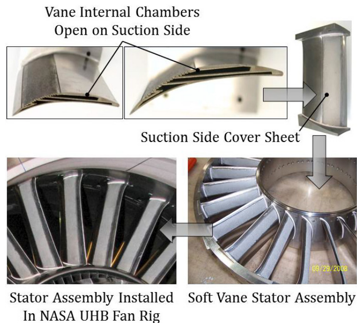
Figure 9.—Soft Vane fan noise reduction concept and its packaging. The hollow vanes internal chambers are tuned to a range of target frequencies and are open on the suction side of the vane. A felt metal mesh cover sheet provides a smooth flow surface.
