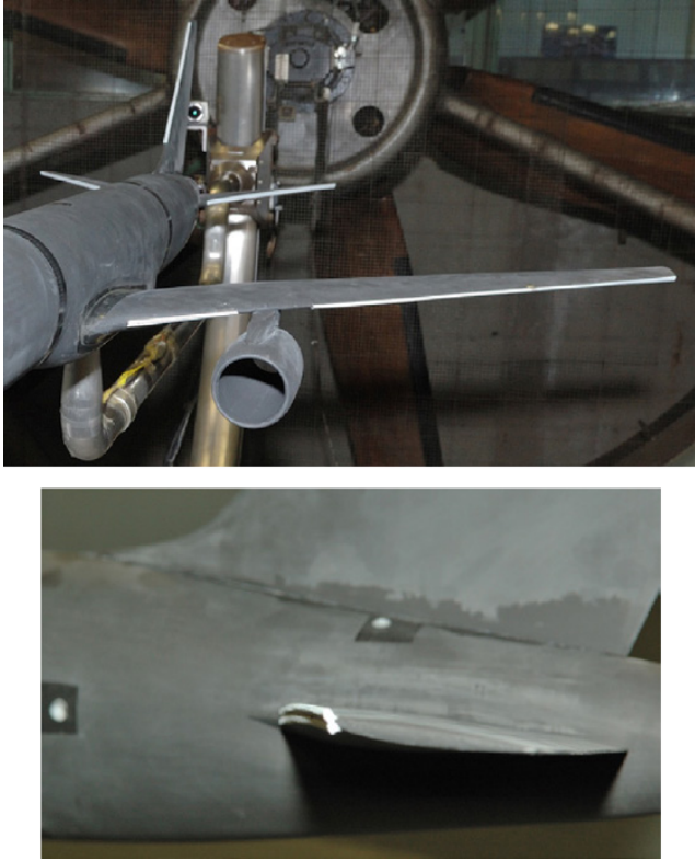
Figure 5.—Artificial ice shapes installed on the 3.5 percent scale GTM, top—wing and tail leading edges; bottom—horizontal tail.
