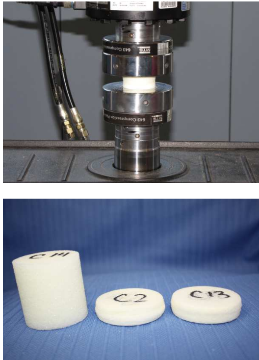
Figure 5 – Foam test setup and foams
