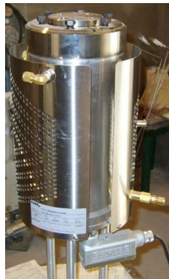
Figure 21. Enhance Test 15 Samples and Sample Holder in an Immersion Chamber
