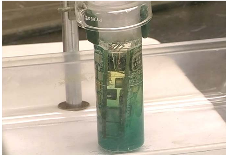
Figure 14. A Non-Standard Screening Test of a Circuit Board Assembly in Hydrazine
