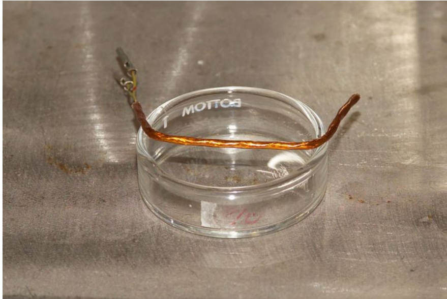
Figure 6. A Beaker Test Vapor Phase Exposure of a Kapton-Insulated Wire with Hydrazine
