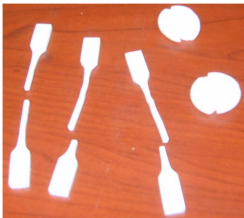
Figure 24. Enhanced Test 15 Posttest Samples following Tensile and Compressive Strength Testing
