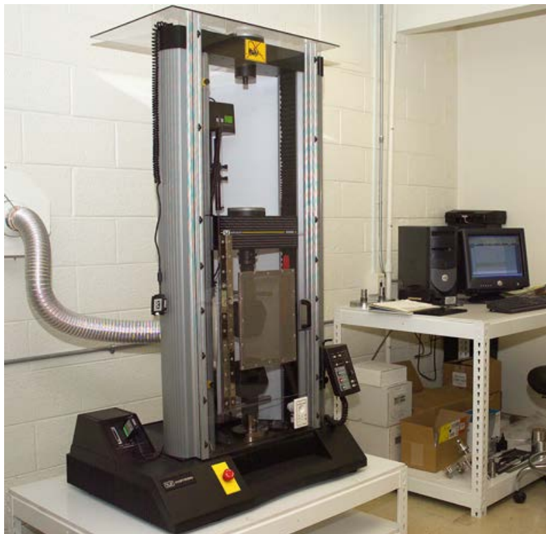
Figure 23. A Universal Test Machine with Local Exhaust Ventilation
