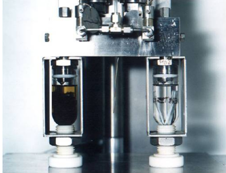
Figure 11. Posttest O-Rings Immersed in MMH
