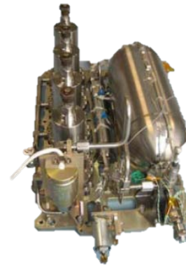
Surrey microsatellite propulsion system
