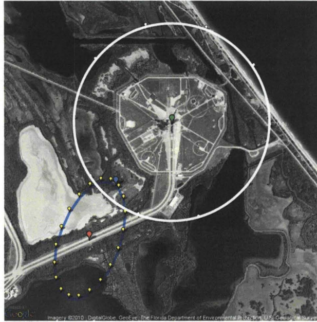
Figure 5. Google Maps visualization of the 99% confidence uncertainty ellipse for nearby lightning strike to Complex 39A on 03 August 2009.
