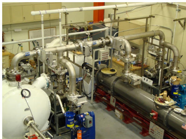
Figure 1. Overhead view of the 5 mm Light-Gas Gun (right) and Flat-Plate Accelerator (white, left) in the Experimental Impact Laboratory at the Johnson Space Center.
