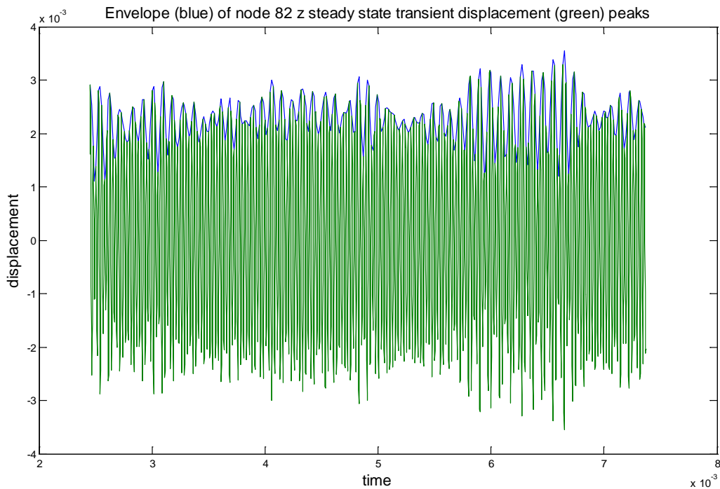
Figure 3. Peak Transient Analysis Response of Highest Responding Node in Beam/Plate Model
