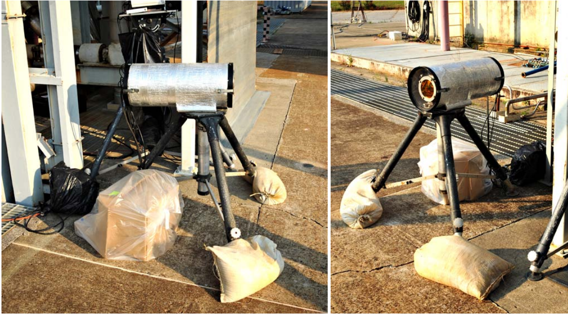
Fig 5 Typical Infrared Camera ASMAT Test Setup. (NOTE: Zinc Selenide (ZnSe) IR window)
