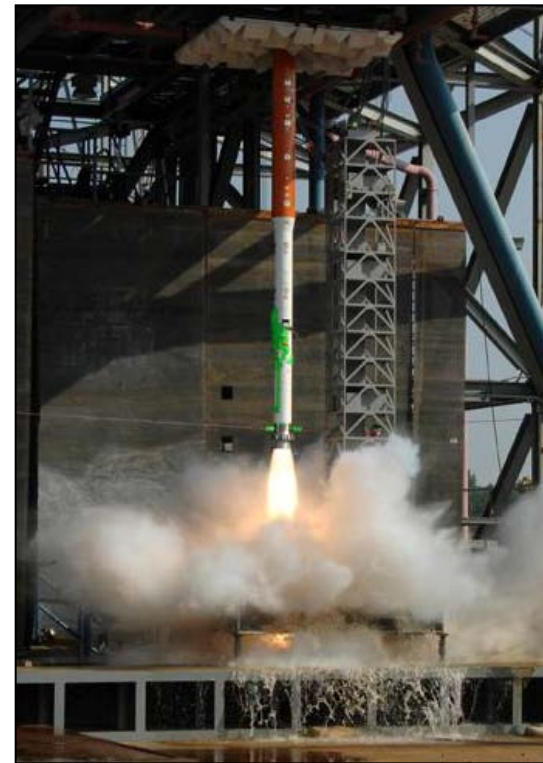
Fig 1. Ares 1-X on the Mobile Launch Pad (MLP) at Kennedy Space Center Launch Complex 39-B and the ASMAT 5% scale model in a lift-off condition at Marshall Space Flight Center East Test Area Test Stand
