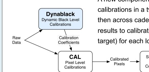
A new component called *Dynablack* performs black level calibrations in a two-step process: first cadence-by-cadence, then across cadences. CAL is modified to use Dynablack results to calibrate science pixels (collateral, background and target) for each long or short cadence.
