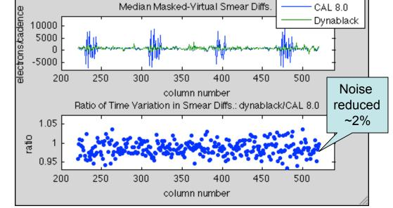
The dynamic black corrected CAL results have not yet been run through the remain pipeline elements, and the direct effect on target pixels is difficult to demonstrate because of the
