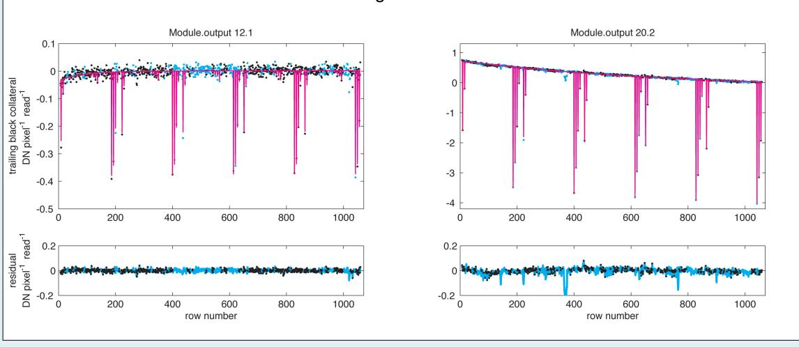
Handling Black-Level Model Coefficients over Multiple Cadences Behavior of spatial fit coefficients vs. time for channels 2.1 and 20.2. An adaptive fitting algorithm
