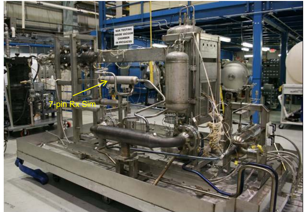
7 Pin Rx Core Sim installed in FSP-PTC
