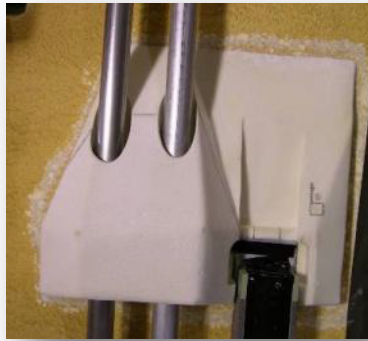
Figure 11. Liquid Hydrogen Tank Ice Frost Ramps
