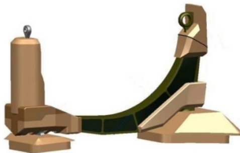
Figure 12. Liquid Oxygen Feedline Titanium Bracket
