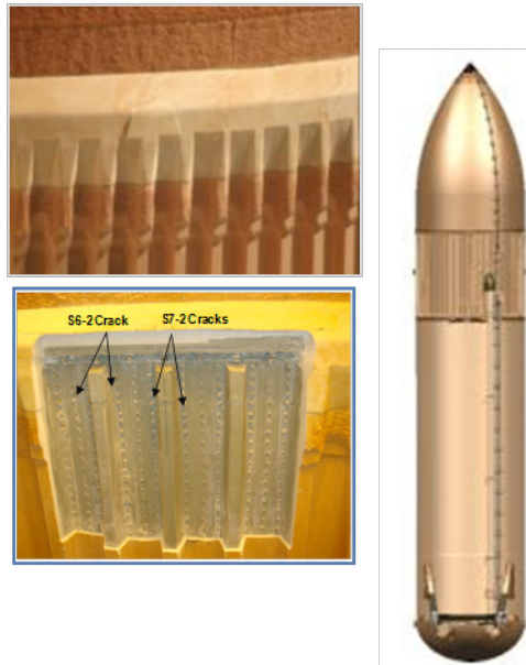
Figure 14. External Tank stringer cracks
