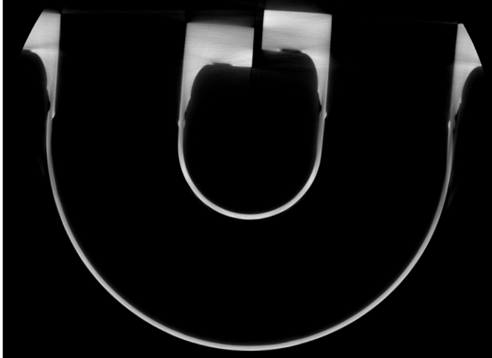
Figure 4: CT Scan through Mid-Section of the Duct
