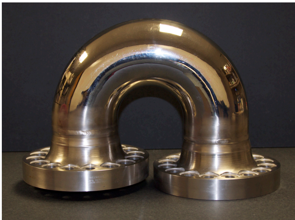
Figure 1: DMLS Duct As Received at MSFC
