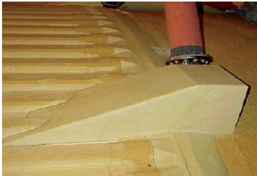
Figure 15: STS-107 Bipod Ramp
