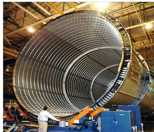
Super Light Weight Tank (SLWT) – Al 2195 alloy
