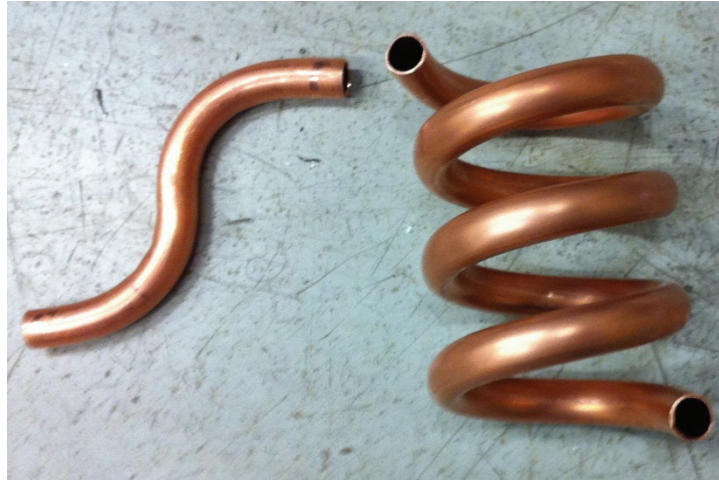
Figure 7. Hand-turned RF heating coil, 3/8-in.-diam tubing.
