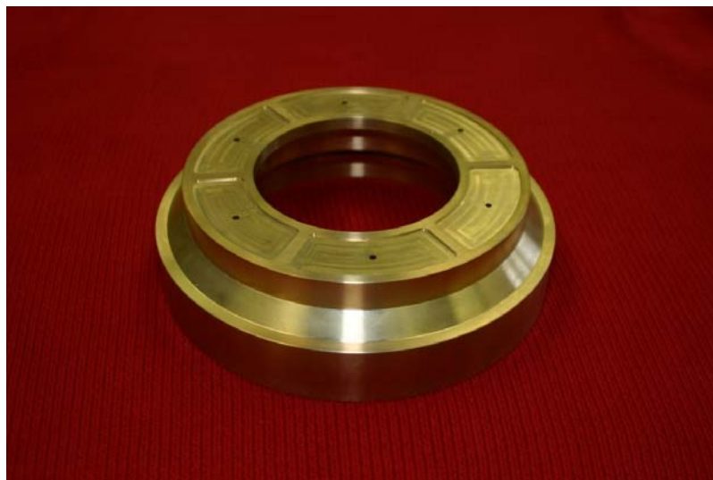
Figure 4 Lower hydrostatic thrust bearing
