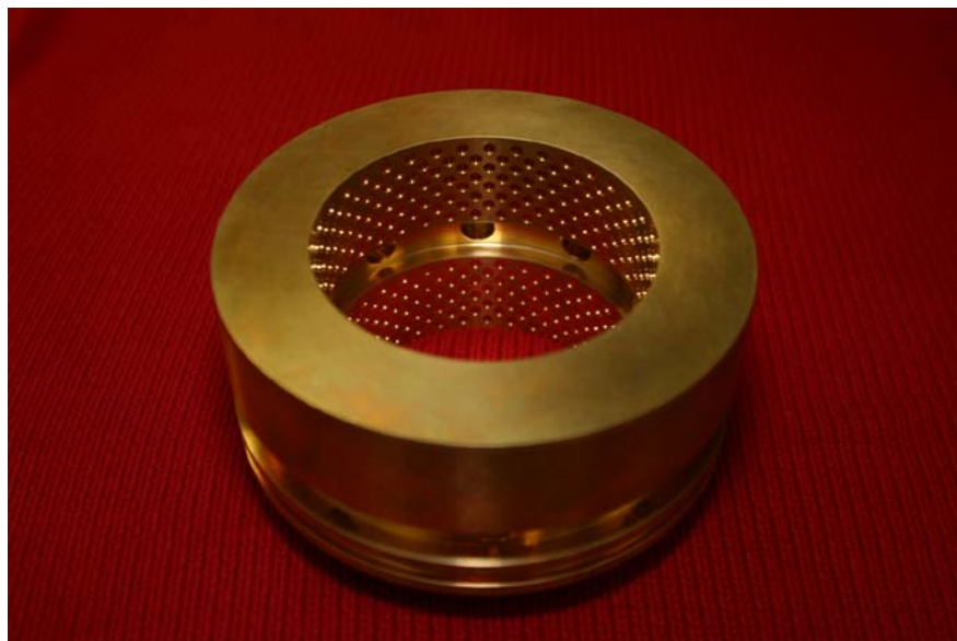
Figure 2 Dual damping seal upper slave bearing
