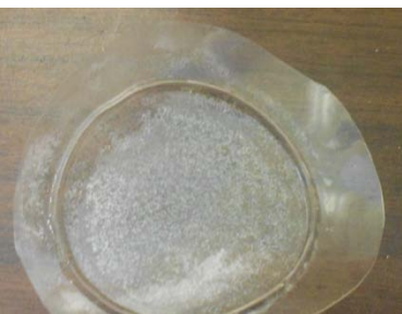
Figure 8. Membrane after long run (Test 4)
