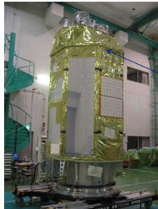
MLI covering the outside of a spacecraft
