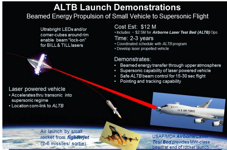
Figure 3.84.—Program 3—Suborbital launch demonstrations using ALTB's multimewatt COIL.
