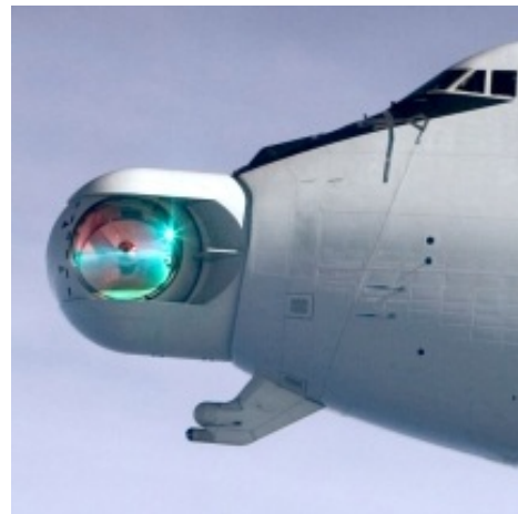
Figure 3.117.—Left: 12-cm-diameter fast-steering mirror for high-power laser applications (image courtesy of ATA; used with permission). A 30-cm-diameter model features >1-kHz open-loop bandwidth, >300 rad/s 2 angular acceleration, <0.2-μm surface accuracy, and ±8-mrad mechanical travel with <10-μrad (2-arcsec) pointing accuracy. Right: YAL-1A ABL prototype in flight, 1.5-m telescope, megawatt-class 1.3-μm laser with undisclosed range .
