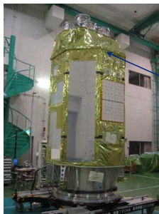
MLI covering the outside of a spacecraft
