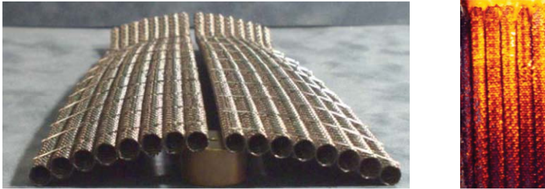
Figure 3.109.—Left: Conformal sections of woven H 2 HX for rocket nozzle cooling. Right: Linear section of woven HX undergoing testing at Glenn. The tests entailed connecting the composite tubes to metal manifolds for the supply and return of 300-to 400-bar H 2 coolant. One side of the panel was exposed to a hydrogen/oxygen combustion plume from a small rocket combustion chamber delivering a free-stream temperature approaching 3,300 K. Panels survived multiple cycles simulating operating conditions of a boost rocket engine (cold-wall heat flux of 20 MW m -2 ), with individual cycles as long as 8 min and cumulative times of 40 min.
