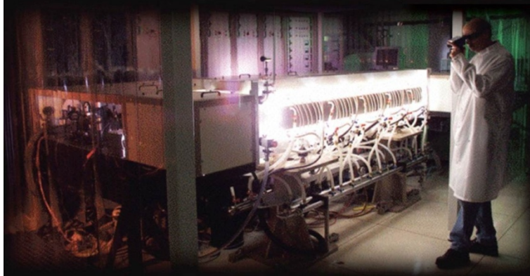
Figure 3.32.—LLNL's 67-kW SSHCL (Ref. 23).
