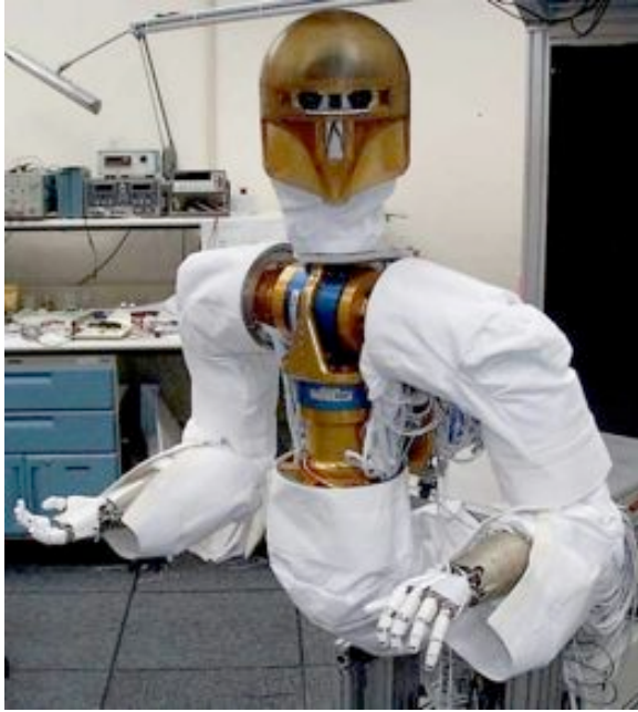
Figure 3: “Robonaut,” a human-equivalent telerobot being developed for EVA at NASA Johnson Space Center
