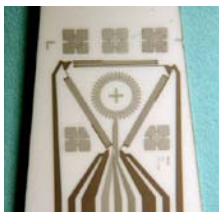
Fig. 2. A thin film multifunctional sensor in the geometry of an off-axis rosette.
