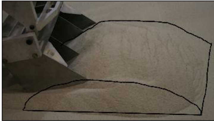
Figure 3. Approximate Soil Volume Outline in Small Bucket for Calculation of Surcharge Mass.
