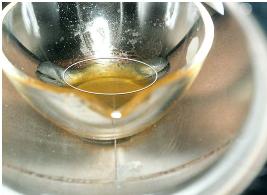
Figure 9. UFORP residue inside vacuum chamber at 10^{-3} Torr after 26 hours
