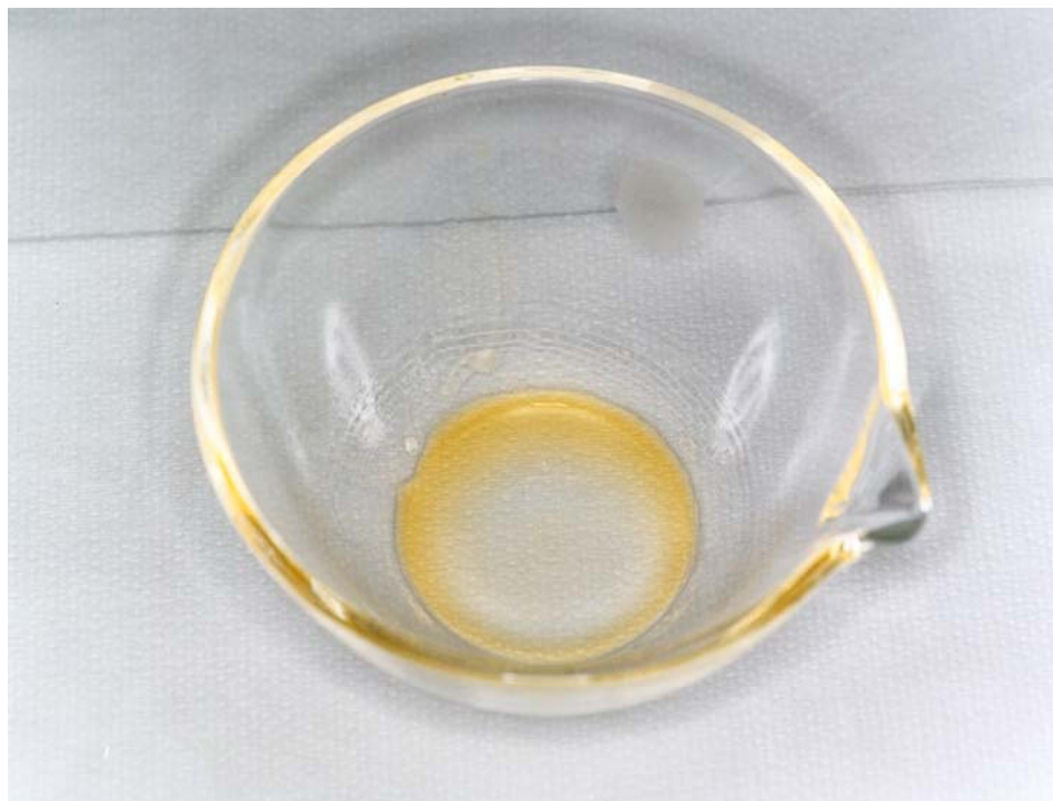
Figure 1. UFORP residue before exposure to 10^{-3} Torr (0.5075g)
