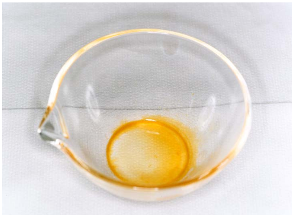
Figure 10. UFORP residue (0.06 g) after 26 hours exposure to 10^{-3} Torr
