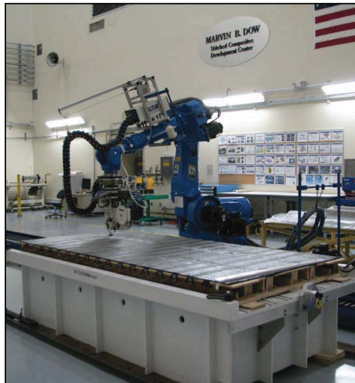
FIGURE 18. SINGLE-SIDED STITCHING TECHNIQUE (DIFFERENT PANEL SHOWN)
