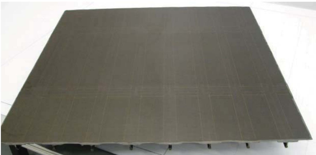
FIGURE 23. CURED SPECIMEN OML SURFACE
