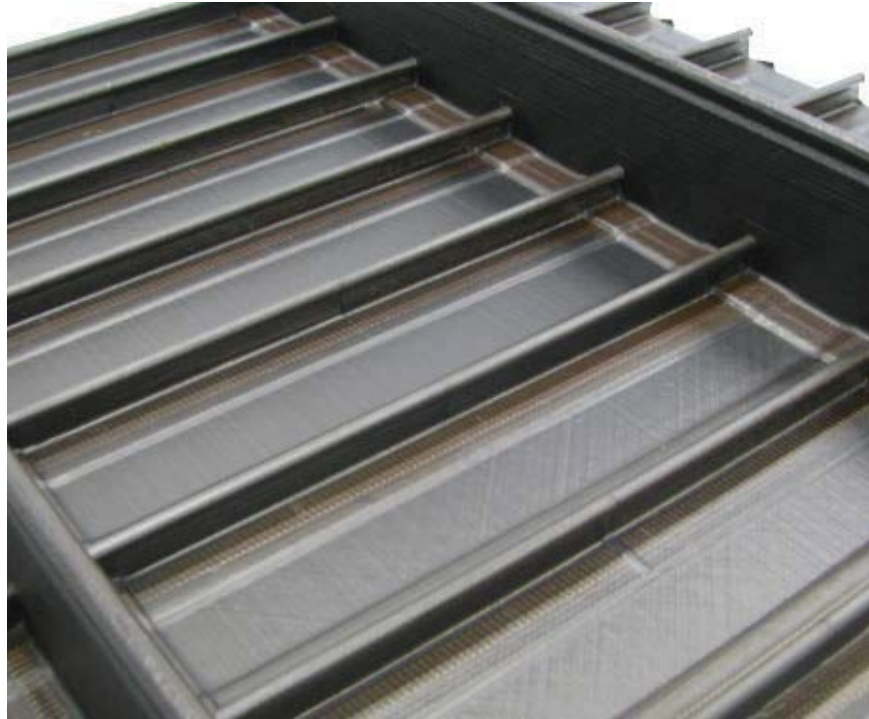
FIGURE 22. CLOSE-UP OF CURED IML SURFACE
