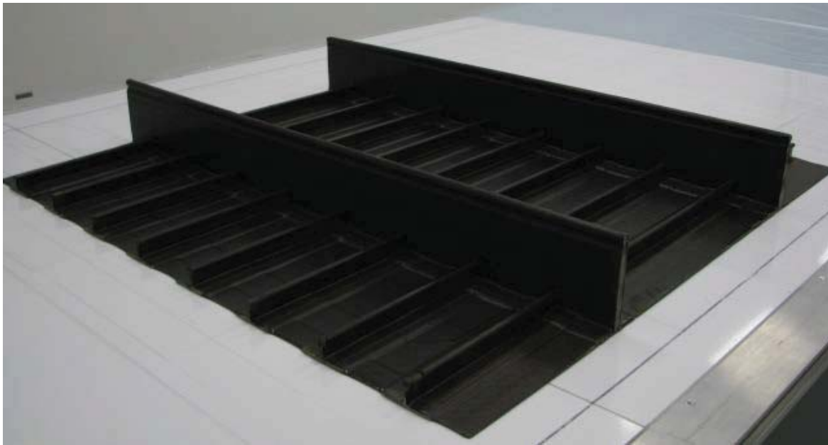
FIGURE 21. CURED SPECIMEN BLANK PRIOR TO EDGE TRIM
