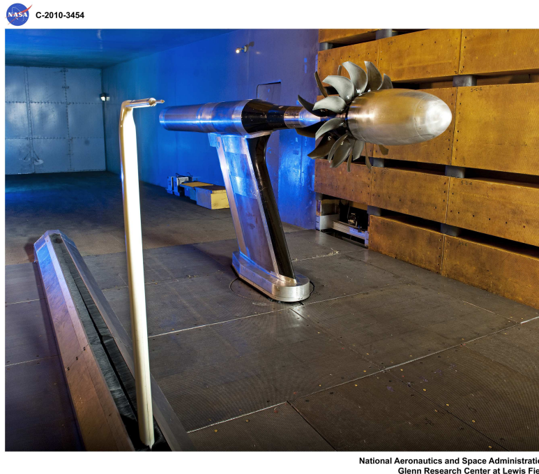
Figure 1: Open Rotor Propulsion Rig in 9x15 Wind Tunnel at NASA Glenn Research Center. NASA Image C-2010-3454.
