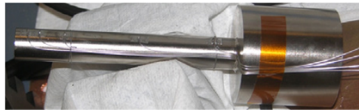
Figure 4.—Thermocouple instrumentation on the GRCop-84 conducting rod.
