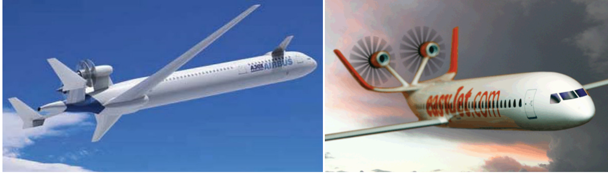
Figure 1.—Proposed Airbus A30X and easyJet ecoJet open rotor airplane candidates having potential empennage shielding benefits (Refs. 6, 7).
