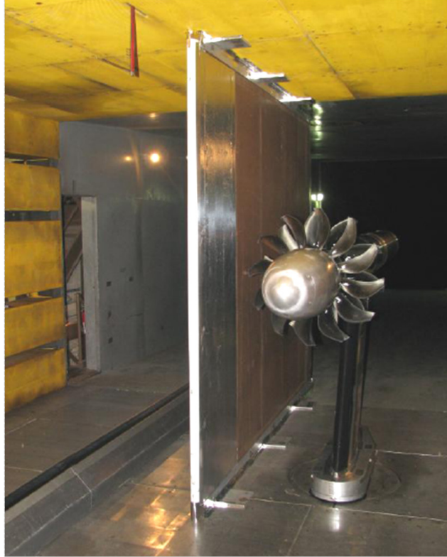
Figure 3.—F31/A31 open rotor test article and “long” barrier wall in the NASA Glenn 9- by 15-ft Low Speed Wind Tunnel. (Photograph courtesy of David Stephens, NASA Glenn Research Center.)
