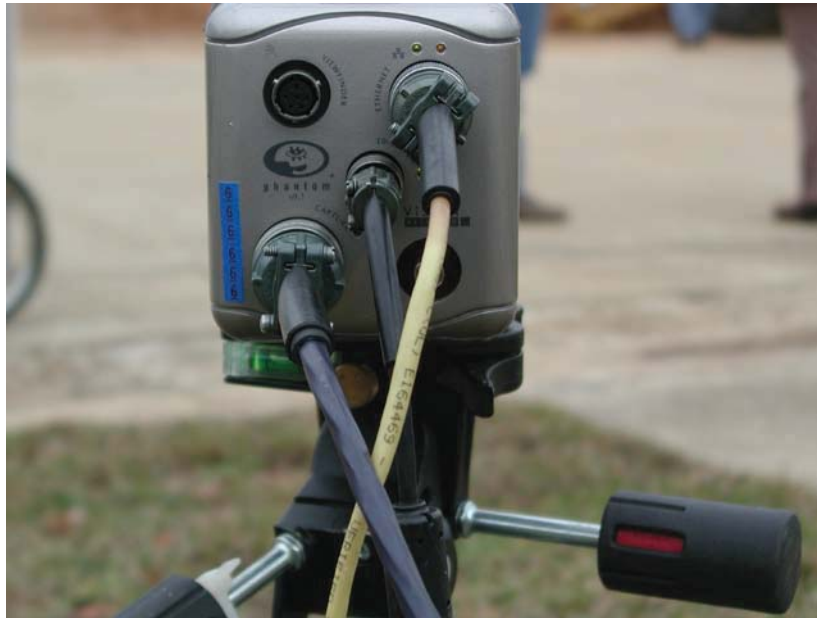
Figure 9. Cable connections for the Phantom camera.
