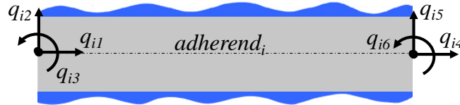
Figure 4.—Boundary conditions for adherend i : prescribed nodal displacements and rotations at x=0 and x=l .
