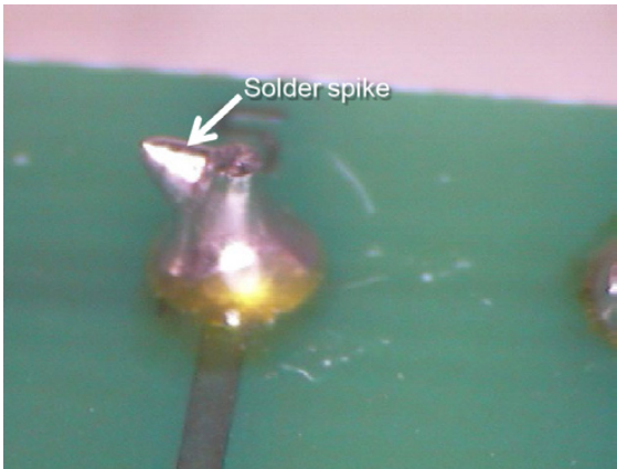
Figure 15.—Example of a solder spike, seen from the soldered fillet side of the circuit board (Eutectic flux cored solder, Joint E5).
