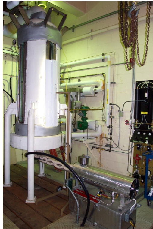
FIGURE 1: The Particulate Aerosol Laboratory: (a) sketch and (b) photograph. Note that in (b), the burner is covered by a pressure housing. The gas (nitrogen or air) from the cold gas supply simulates the atmosphere, and the burner exhaust simulates aircraft engine exhaust.
