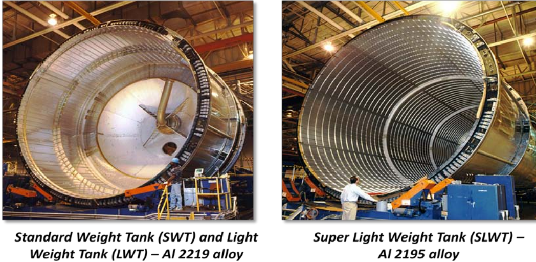
Figure 5: Comparison of SWT / LWT to SLWT LH2 Tank Barrels
