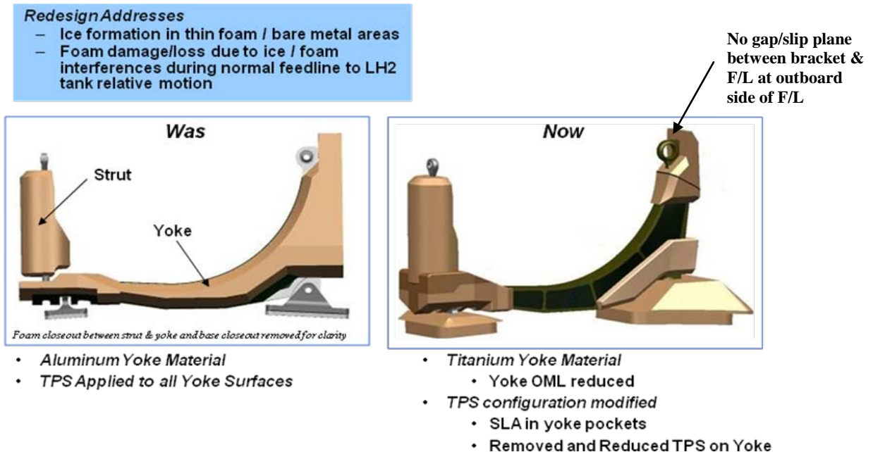
Figure 22: LO2 Feedline Brackets Before and After Redesign
