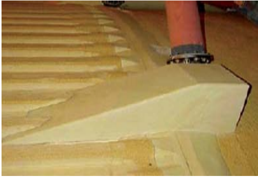
Figure 15: STS-107 Bipod Ramp
