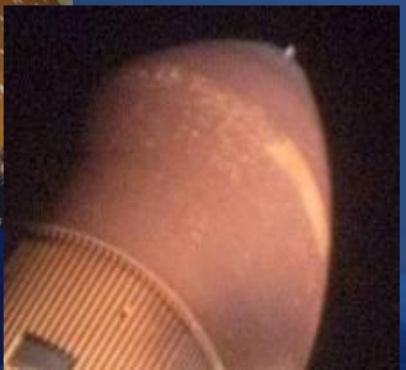
ET-124 Damaged by Hail Storm on Pad
