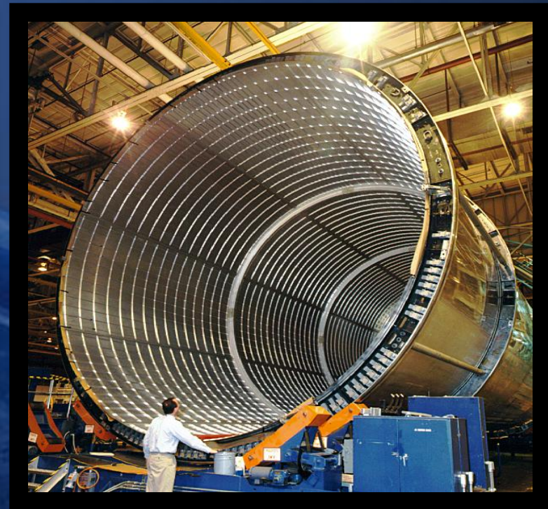
Super Lightweight (SLWT) – Al 2195 alloy
