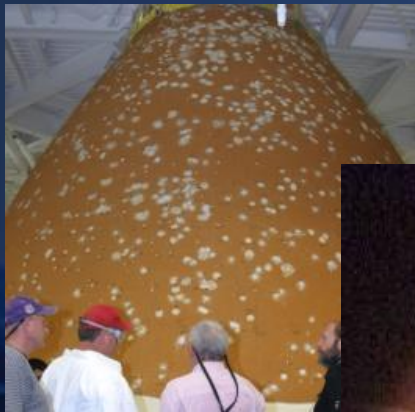
ET-124 Damaged by Hail Storm on Pad
